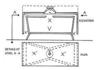
Patent for a double bass reflex <u>loudspeaker enclosure</u> design intended to produce infrasonic frequencies ranging from 5 to 25 hertz, of which traditional <u>subwoofer</u> designs are not readily capable.
